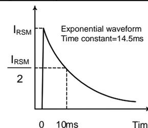
Figure 1.  $I_{RSM}$  waveform
