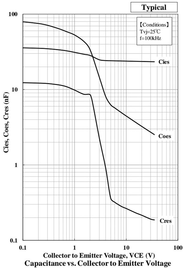
Capacitance vs. Collector to Emitter Voltage
