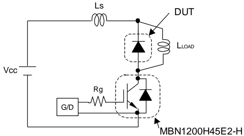
**Fig.1 Switching test circuit**
