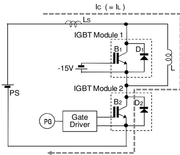
Fig.3 Current flow in ON-state of B2
