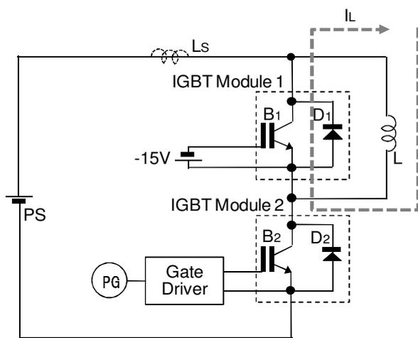
Fig.4 Current flow in OFF-state of B2
