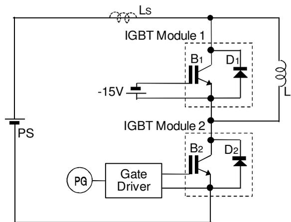
Fig.1 Half-bridge circuit
