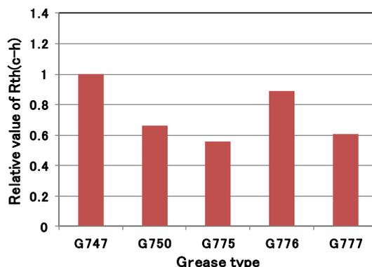
Fig.5 Thermal resistance comparison among grease types
