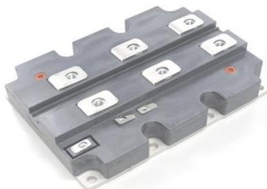
Fig.2 IGBT module used for measuring thermal resistance
